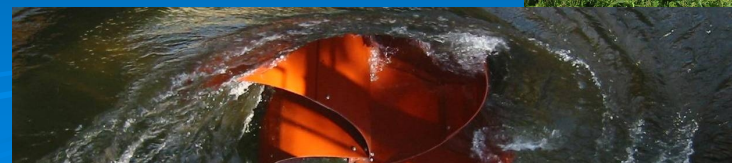
↑ The water vortex turbine extracts the rotation energy from the gigantic water vortex and powers a generator.
