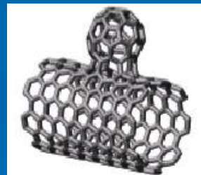
↑ A Nanobud combining a nanotube and a fullerene. Nanobuds are good field emitters.
