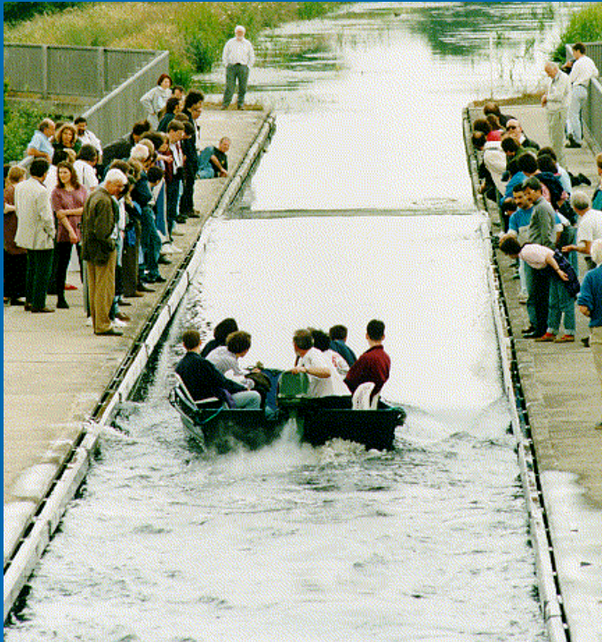
↑ Soliton on the Scott Russell Aqueduct on the Union Canal near Heriot-Watt University.
