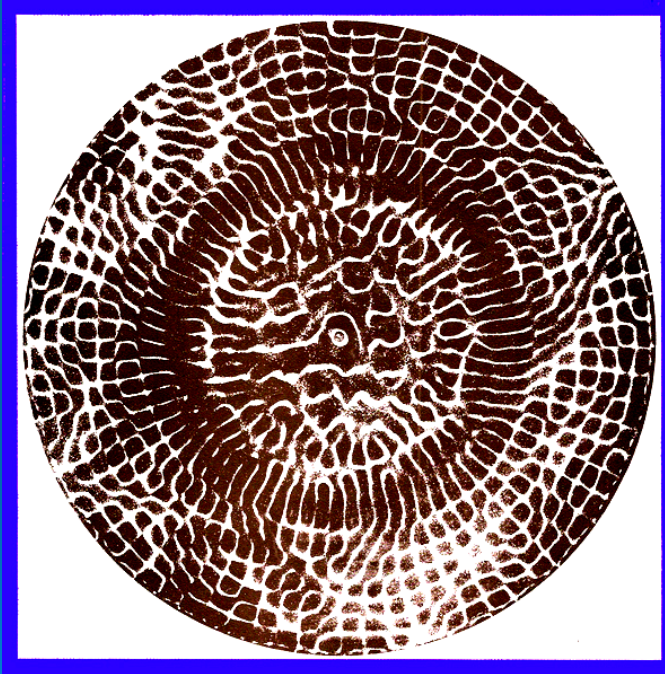
↑ Plate = 50 cm Frequency = 6,250 Hz.
