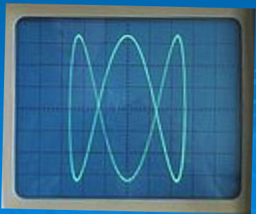
← Lissajous figure for the octave on an oscilloscope.
