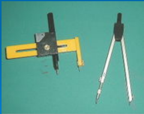
Left: beam compass Right: school compass
