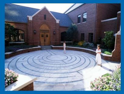
↑ St. Paul's labyrinth design (1996) was built using pre-cut arcs and geometric sections of Tennessee Bluestone and Indiana Limestone. Pre-cut with abrasive waterjet, the sections were palletized and delivered to the site.
